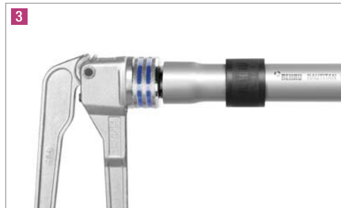
3. Expand the pipe end
